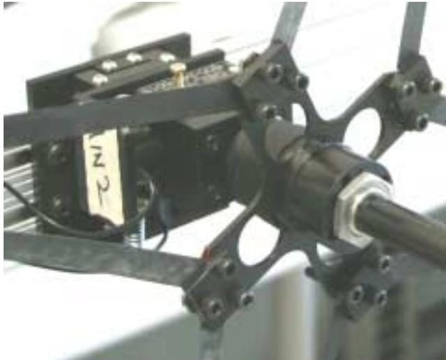
**Figure 29. Load Cells, Ball Slides Opposite the Motor**
