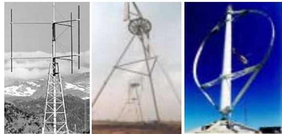
Figure 4b. Three Vertical Axis Windmills
