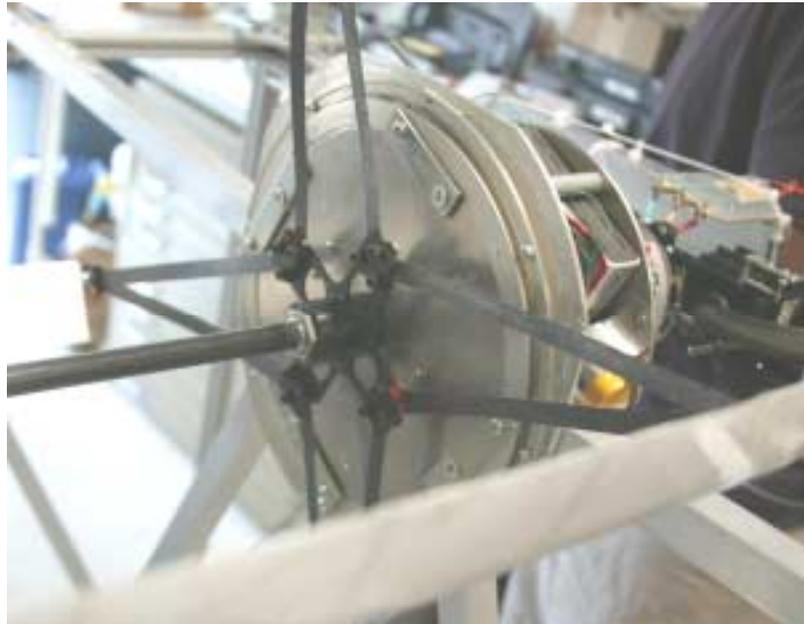
**Figure 33. Tension Struts at Motor End of Rotor**
