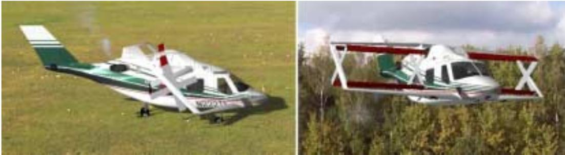
The cyclogyro is one of the most heavily studied subsonic aircraft concepts that has never flown. It is based on the principle that airfoils arranged with their spans parallel to an axis of powered rotation normal to aircraft direction of flight can be controlled in pitch so as to provide lift and/or thrust in any direction within a vertical plane, as shown above. This is not a new concept, and its potential for VTOL to high speed flight has long been recognized.
