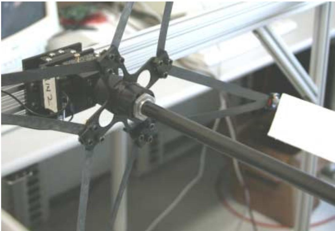
**Figure 30. .007" Thick Tension Struts and Hub.**
